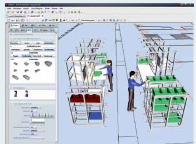
Multiple workstations are linked to form a production line that follows lean production principles
